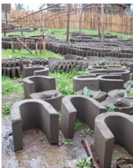
Above: A factory in Ethiopia producing concrete stoves.
